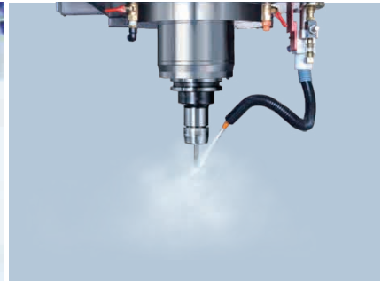
Oil Coolant System
